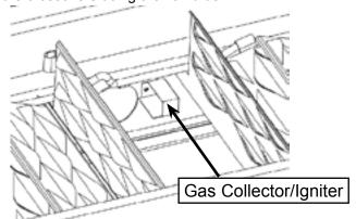
With the louvers raised, brush the ashes from the gas collector/igniter. You will need to raise each pair of louvers and clean the ash from the grill. Note: The ashes can be brushed into the bottom of the grill for removal.
